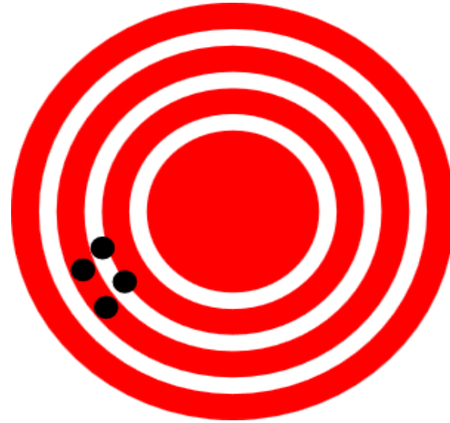
準確度低，精密度好，真實性差 Low accuracy, good precision, poor trueness
